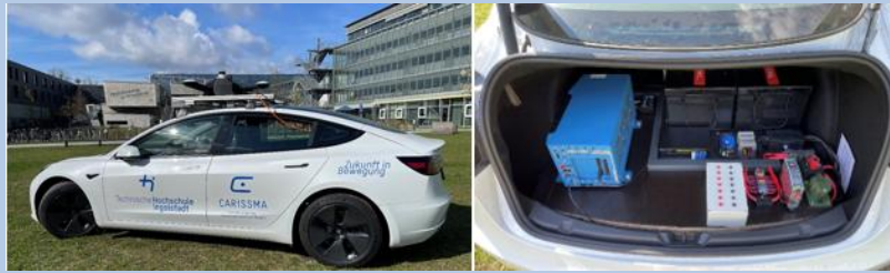
Fig. 3: Setup of the Tesla Model 3 research vehicle with additional environmental sensors (cameras, radar, lidar) mounted on the roof and the remaining equipment (car PC, power supply, wiring, ...) installed in the trunk.
