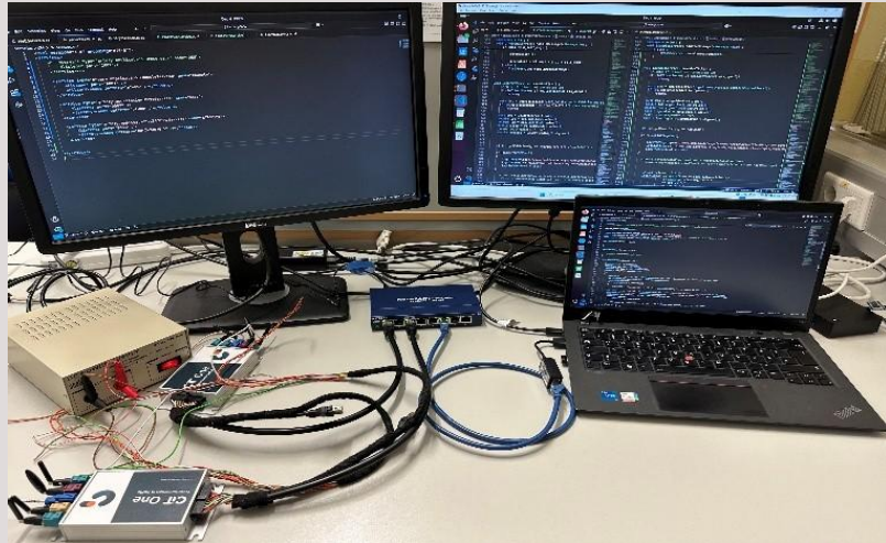
Fig. 2: Test Environment to validate Car2X applications for PTWs.
